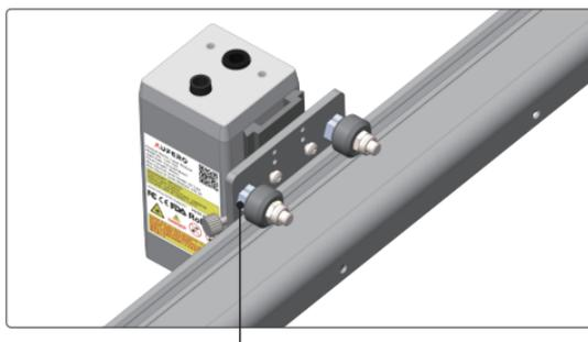
Use a wrench to adjust the eccentric nut to adjust the gap between the wheel and the profile
