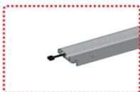
Thread the Y-axis motor cable inside the Slideway of Left Y-axis
