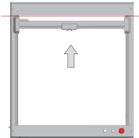
Push the X-axis assembly to the rear limit point
