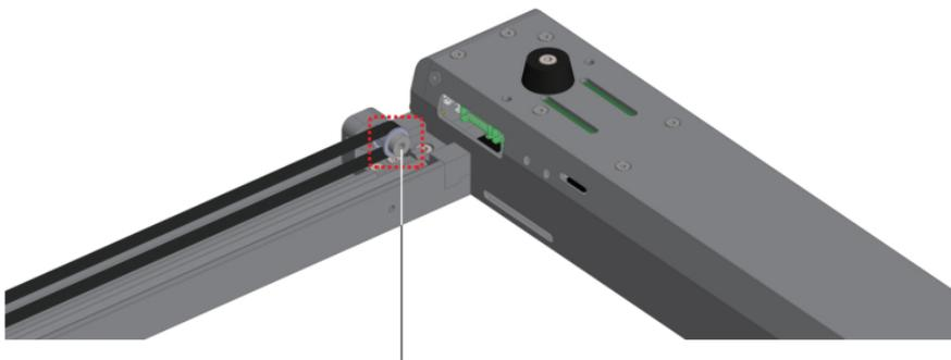
After the timing belt is tightened, use a 3mm Allen key to lock the idler pulley assembly
