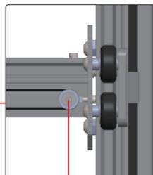
Loosen the screw, adjust the tightness of the belt, and then retighten the screw to fix it
