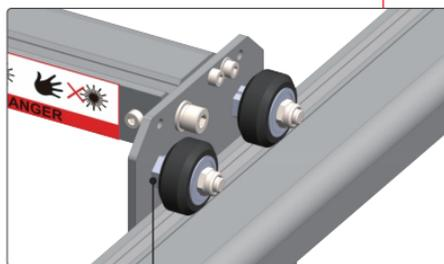
Use a wrench to adjust the eccentric nut to adjust the gap between the wheel and the profile (same on the other side)
