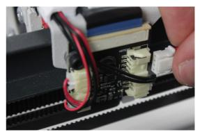
**11.** Place and adjust the zip tie, cutting off the excess.
