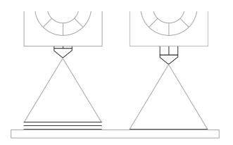
The Sigma automatically corrects the offsets when printing in Duplication/Mirror modes. However, this correction distorts the first layer of the model by repeating it as many times as needed.
