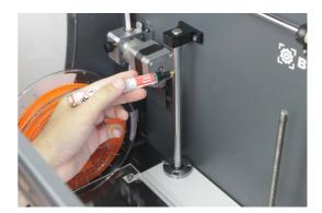
**3.** Apply the lubricating oil pencil along the Z shaft bars, making sure that it does not drip.
