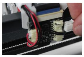
10. Remove the old hotend and place the new one, connecting it at the back of the toolhead carriage.
