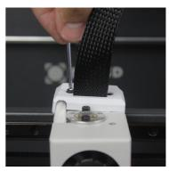
13. Insert the teflon tube until it stops, making sure it is well placed. Put back the black clip.
