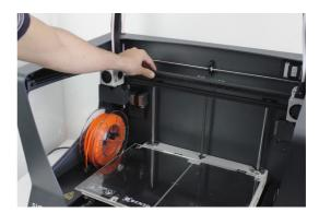
**8.** From the center towards the ends of the linear guides of the X and Y axes, remove dirt with an absorbent paper or a cloth.
