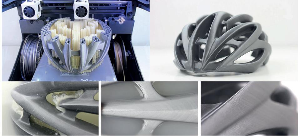
After support removal and depending on the material used for the print, there is a big range of post-processing techniques that can be applied to the part:
