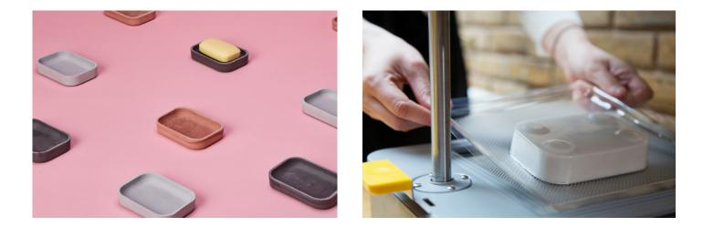
"By 3D printing a master model and creating a 3D two-part mold using the FormBox, we were able to efficiently create a set of soap dishes that fitted the clients needs perfectly"
